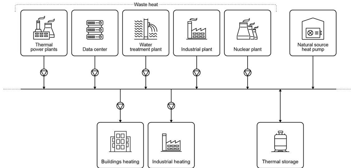
**Heat pumps can play diverse roles in district heat networks through connections to primary networks, secondary networks and to substations.**
