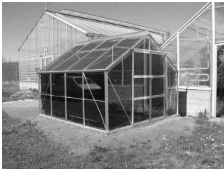
Figure 5: The Greenhouse test hut, designed for testing wood against discolouring organisms
