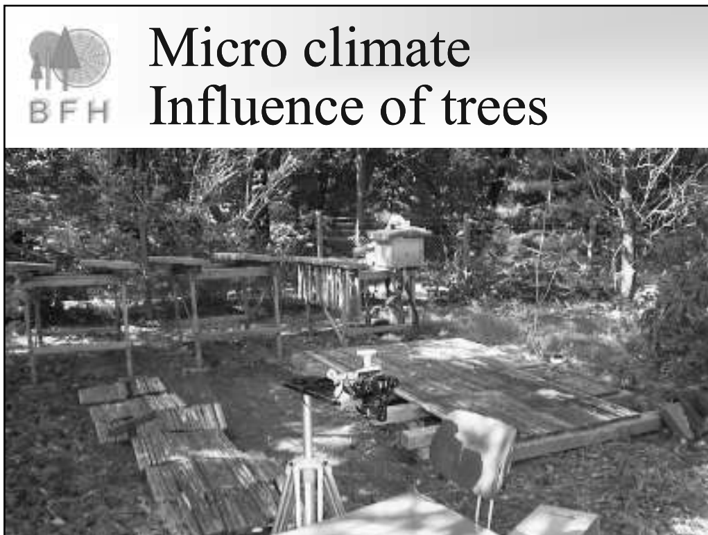
Figure 2. Test site in Hamburg close to trees, showing a double layer deck which is opened for evaluation after 4 years
